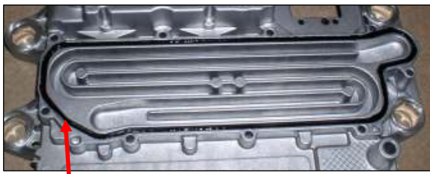
Bottom section with channel filled with sealant
